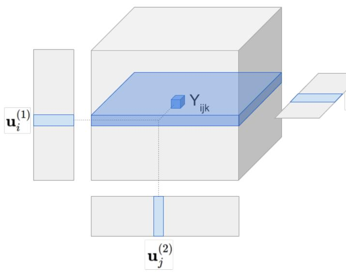
Tensor model predicts Yhat [i, j, k] by multiplying all latent vectors together element-wise and then taking the sum along the latent dimension (figure omits the global mean).
